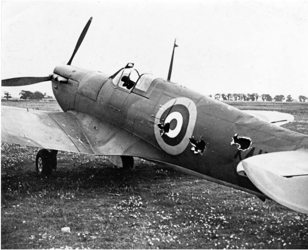
Another view of the same aircraft, illustrating the potency of the Bf 109s 20mm cannons. (Fighter Command Station at War)
