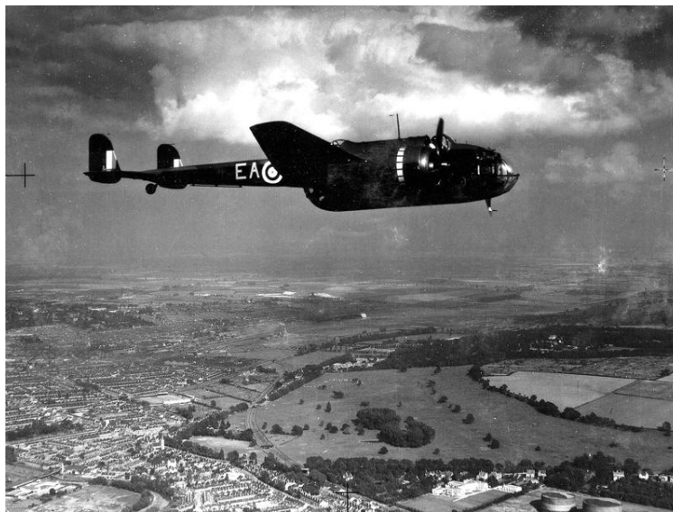
An air to air shot of a 49 Squadron Hampden, showing of its unusual shape, narrow and deep crew compartment and thin tail, very small rudders. The Hampden ended up being known by many crews as the 'Flying Suitcase'.
